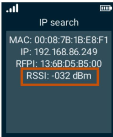
As you walk around with the wireless handset, the RSSI will automatically update onscreen with the signal strength for that area.
